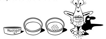
Make your own sieve by making holes in the bottom of a plastic margarine tub. The holes must be big enough to let the particles of the smallest solid through, but too small for the bigger bits of the other solid.
